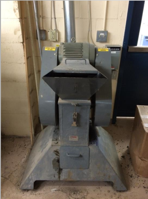
CIR or FDR Cores are cut down to a manageable size and crushed to a target grading
